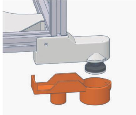
Place the pins that serve as a stop to the leading edge of the wing in its position
